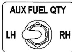
The actual fuel quantity in the respective tank (LH/RH) is the sum of the central indication and the corresponding indication on the left or right side.
